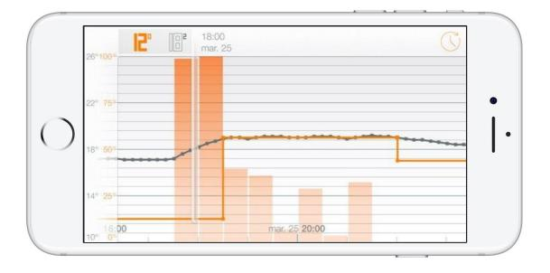
**Note:** The use of the PID algorithm is automatically suspended for all setpoint temperatures less or equal to 14°C. The hysteresis algorithm is then reactivated: it is indeed useless to switch the heating more frequently to improve comfort when an economic setpoint is activated. The PID algorithm is reactivated as soon as the setpoint goes above 14°C.
