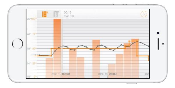
**Please note:** When the setpoint is changed, the Thermostat responds instantly to the new setpoint without needing a threshold to switch the heating on or off.
